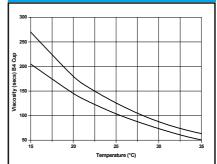
Comparison graph of Temperature vs Viscosity using a B4 flow cup. The graph, which shows the upper and lower limits of operating specification, is a small-scale version. Full-scale curves are available on request and these should be used as a guide to maintain and control tank viscosity. A tank sampling service is available on request.
