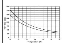
Comparison graph of Temperature vs Viscosity using a B4 flow cup. The graph, which shows the upper and lower limits of operating specification, is a small-scale version. Full-scale curves are available on request and these should be used as a guide to maintain and control tank viscosity.
