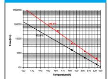
Thermal Endurance has been carried out on Helical Coils & Twisted Pairs to ASTM D3145 and D3251 respectively (as recognised by Underwriters Laboratories).
